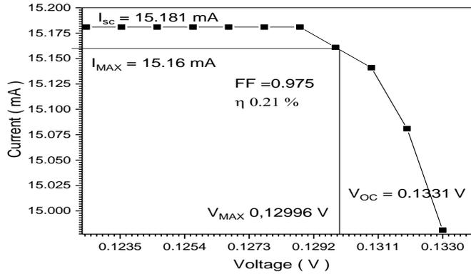
Fig (2) I–V Curves of Rhodamine B Dye
